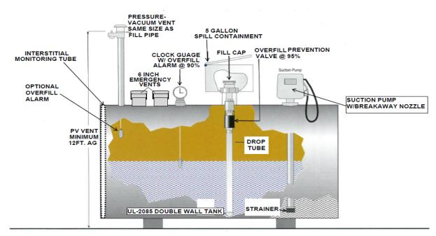
Aboveground Bulk Tank with Remote Pump(s)
